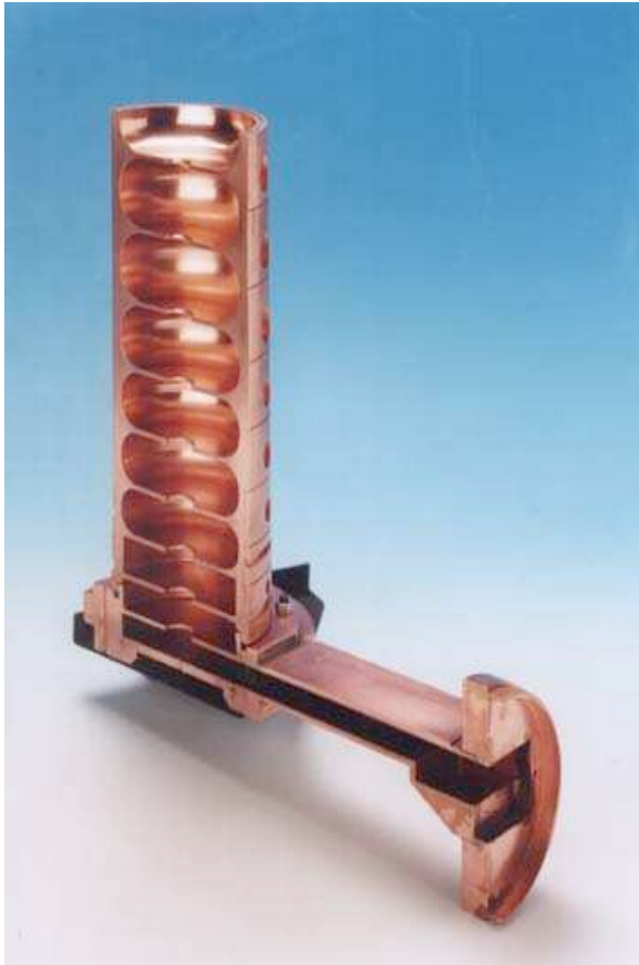
Short section - TW accelerator
