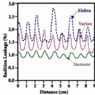
Fig. 1. Leakage patterns for the major MLC collimators. From: Huq MS, Das IJ, Steinberg T, Galvin JM (2002) A dosimetric comparison of various multileaf collimators. Phys Med Biol 47(12):N159-N170.
