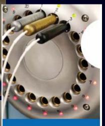
Ergonomic turret with quickconnects The turret offers ergonomically designed quick connects with unique keying possible on channels 1-4, and the electronic locking system with connection verification – both unique to VariSource.
