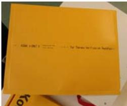
Since there is no conversion of x rays to light photons as in diagnostic films, the films need not be removed from its envelope.
