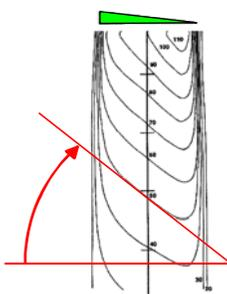
The diagram shows a cross-section of a wedge filter. A red line indicates the beam central axis, and a red arc indicates the angle between this axis and the 50% isodose line. The isodose lines are labeled with percentages: 100, 90, 80, 70, 60, 50, 40, 30, 20, 10.
