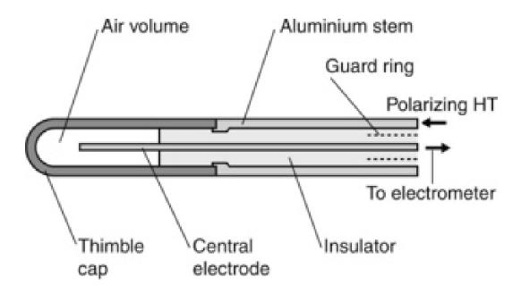
• Stem effect is caused by interactions of radiation with air near the chamber end, or with dielectric in the chamber stem or cable.
